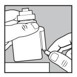
Break the seal on the vent tube to allow air flow. Tab can be completely removed or bent enough to open vent and remain attached.
